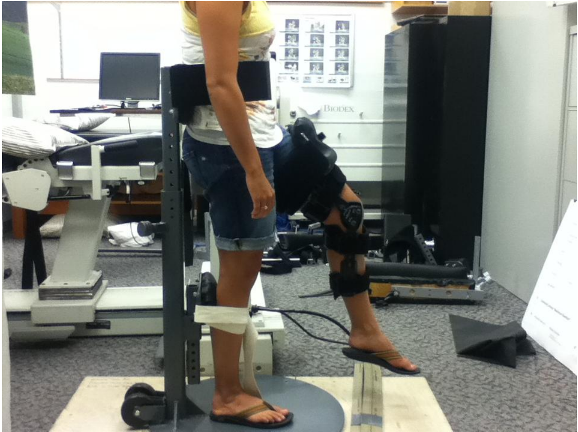
Figure3.1. Experimental setup for hip flexion and extension motion testing.
