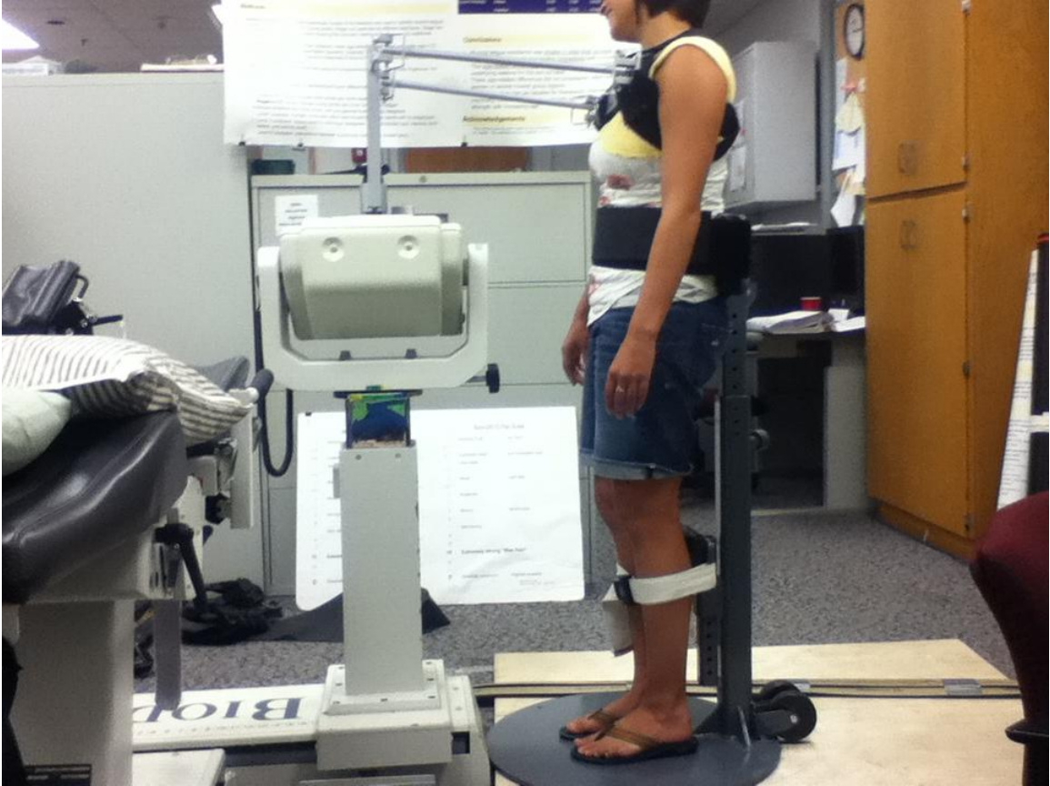
Figure 3 .3. Experimental setup for trunk rotational motion testing.
